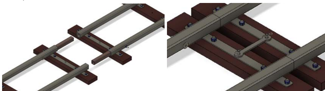
CAD render of joining of Jubilee Track panels.
