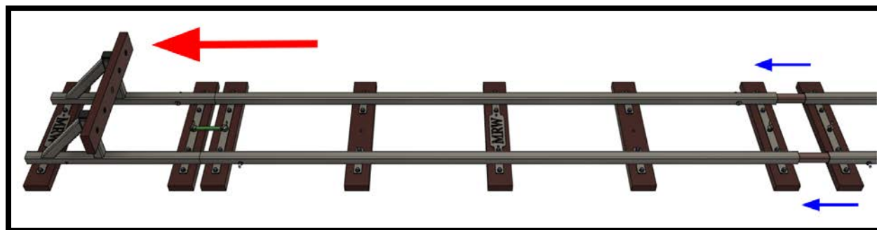
Above Diagram: Buffer stop connected to track panels with “Track Panel Tie Bar”.
